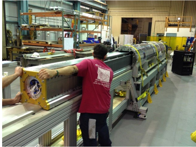
LHC Nb 3 Sn superconducting Quadrupole magnet
